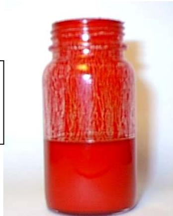
Flocculated system where the pigments separate and formed an un-homogenous
