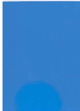
A more stabilized system. There is still some small white rub out (color turn lighter) where the white based is not well stabilized. However you can notice that the rub out area has different color tone, a high possibility that both pigments are still not well stabilized.
