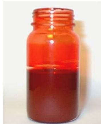
Stabilized system where the pigments dispersion formed a homogenous film
